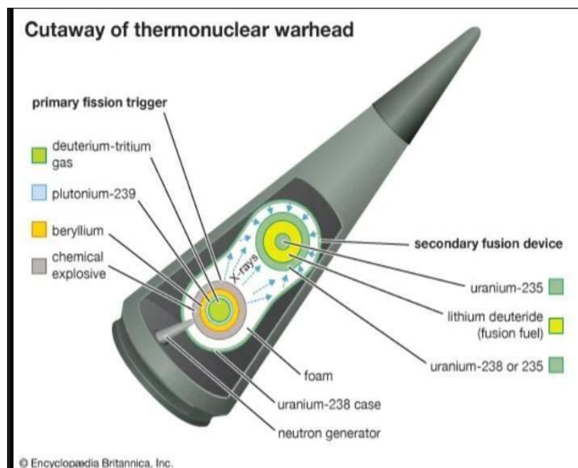
Figure (16): Cross-section of a thermonuclear warhead.
