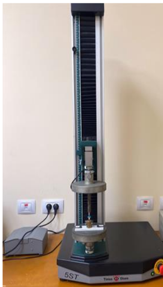
Figure (3): Universal testing machine used to measure the fracture resistance (Tinius Olsen)
