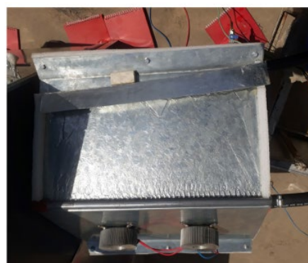
Figure 21 External Condenser Closeup [41].
