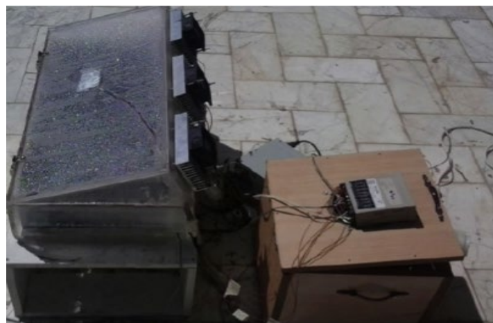
Figure 8 Double Condensing Region TEC-Assisted Solar Still [28].
