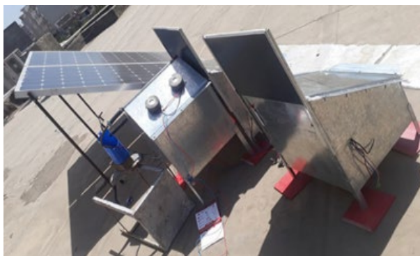
Figure 20 TEC-Equipped Solar Distiller with Nano Silver and External Condenser Augmentations [41]
