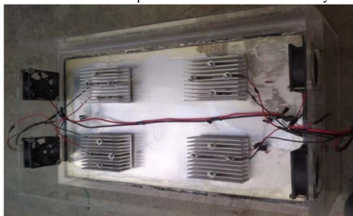
Figure 4 TEC Assisted Double-Slope Double-Story Solar Still [24].
