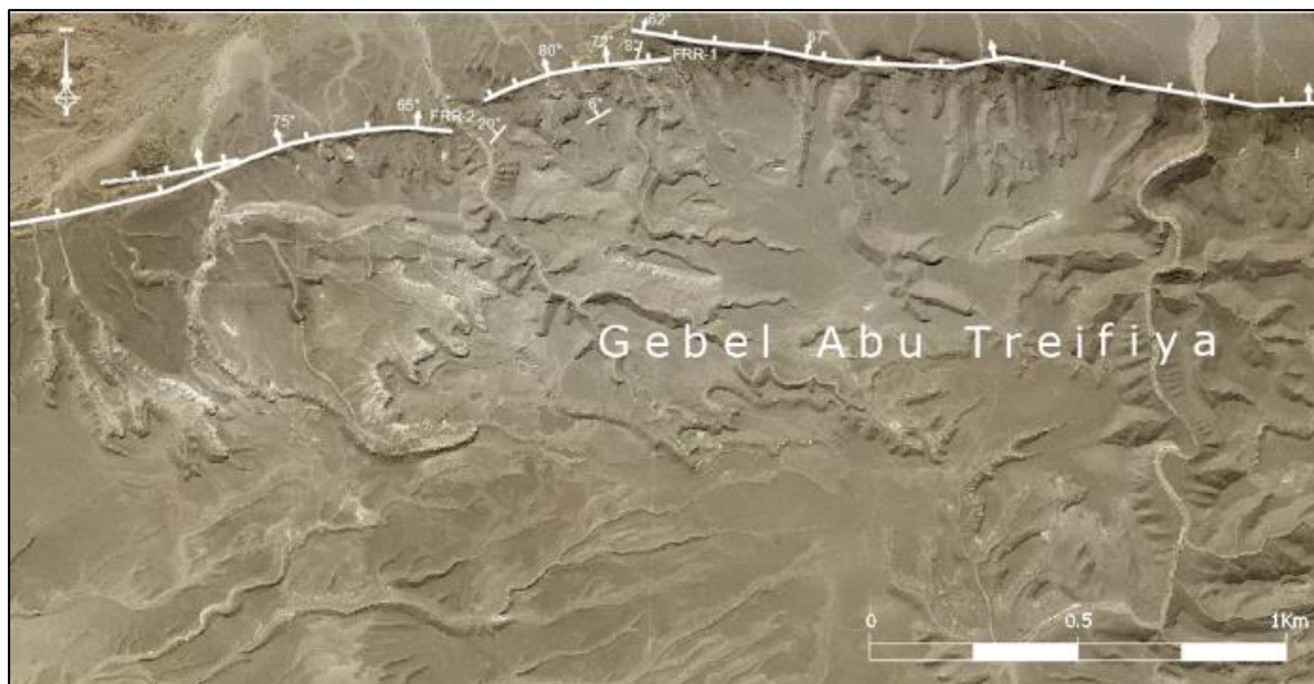
Fig. 19. Satellite image showing relay ramps (FRR-1 and FRR-2) between two en echelon E-W oriented normal faults bounding the northern side of Gebel Abu Treifiya.
