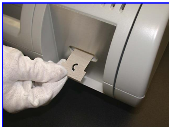
Figure 3. Inserting sample trap into disrober.
