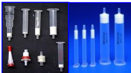
Figure 1. Solid-phase extraction technique SPE column.
