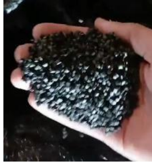
Figure 5 . polypropylene pellets (PP) with 20% fiber glass
