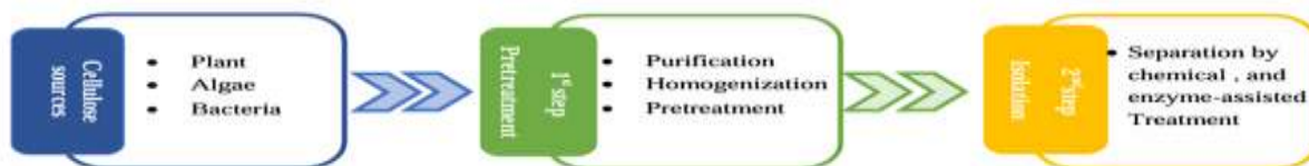
Figure 3. Process flow for synthesizing CNCs from various sources [6].
