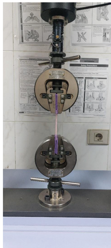
Poly methyl methacrylate specimen positioned on universal testing machine measuring the tensile strength.
