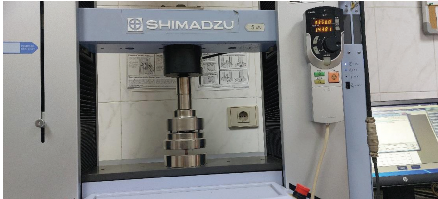
Measuring the compressive strength for poly methyl metha acrylate specimen positioned on the universal testing machine.
