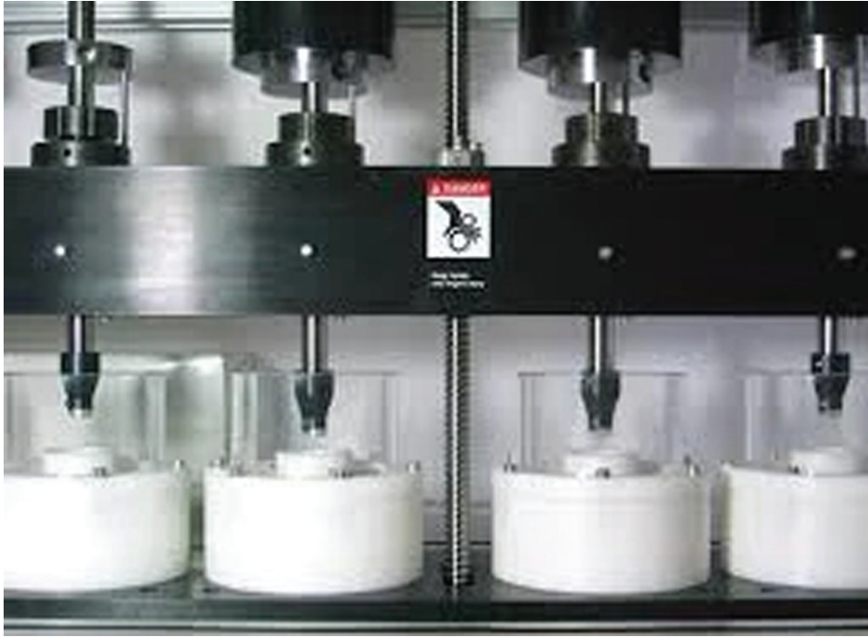
Chewing simulator used for wear simulation test (ROBOTA Co.).
