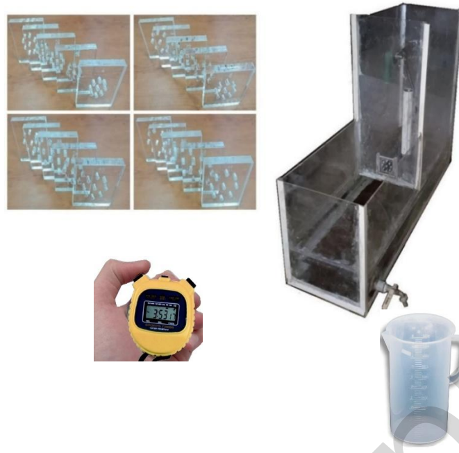
Fig. 2: Real photo of the physical model and orifice plates
