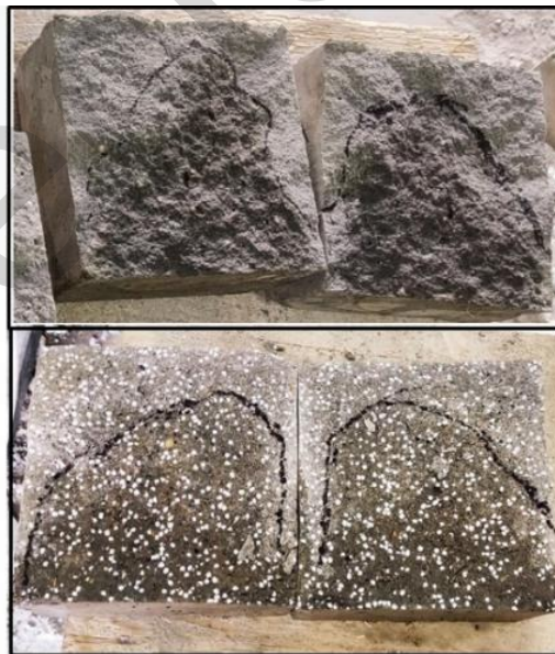
Fig. 11: Water Penetration Resistance specimens after test
