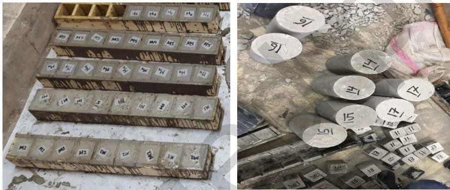
Fig. 4: Fresh Concrete in Molds.
