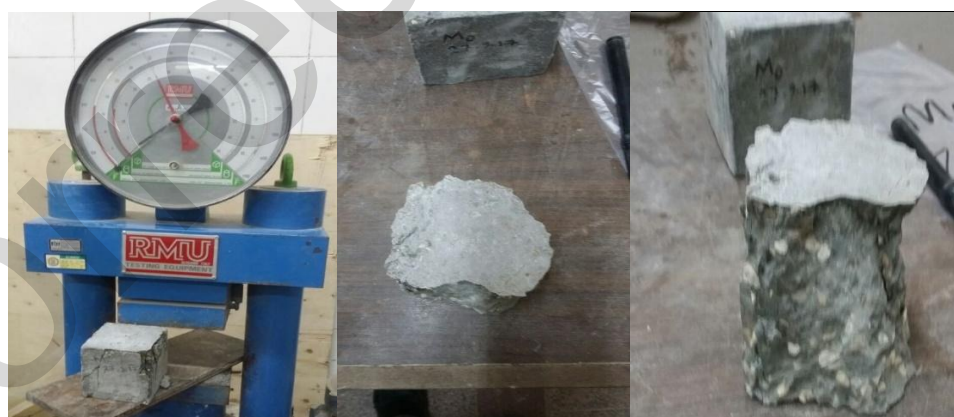
Fig. 7: Hydraulic Testing Machine Used in Compressive Strength Test.
