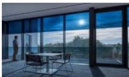
Fig. 4: switchable electric glass [Spendlove, T. (2016). Breathing Bio Metal Regulates Building, erging-materials-thermo-bimetals Temperature).
