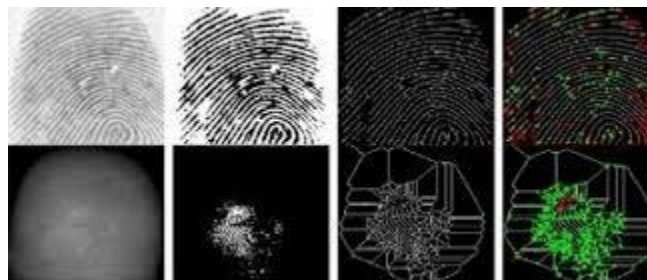
Figure 5. Shows fingerprint binarization, thinning and false minutiae removal.
