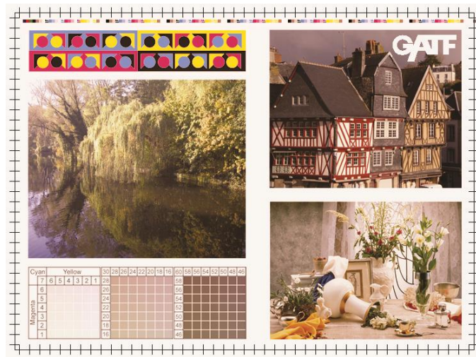
Fig. (5) Weak Cyan was appeared in printed sheet
