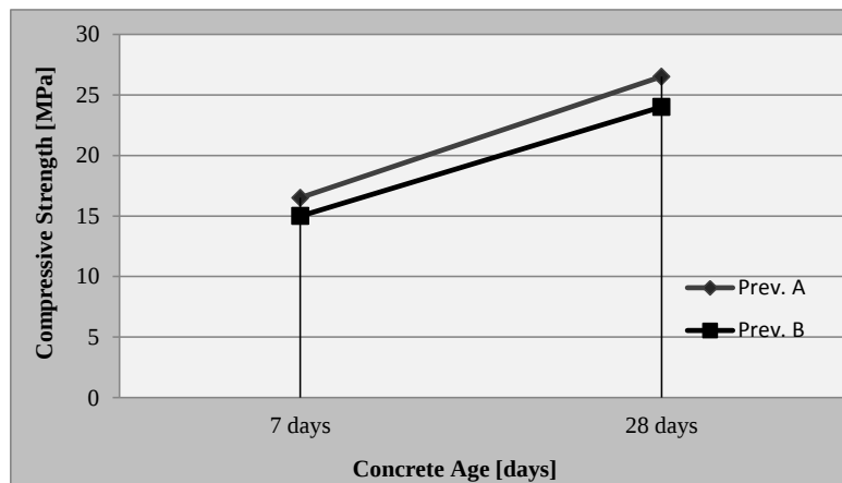
Figure 4. Compressive Strength Evaluations
