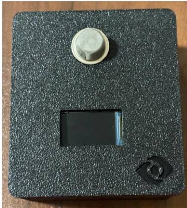
Fig. 3: Updated prototype of the breath ketone detection device.
