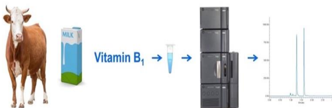
Fig. 3: Graphical abstract of HPLC determination of thiamine in bovine milk 14 .
