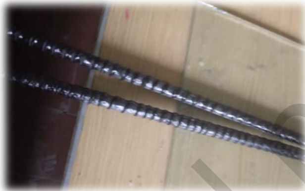
Fig.6: Final production of Roughened Hybrid-bars
