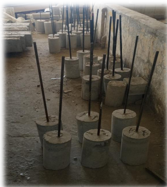
Fig. 17: Samples of pull out test
