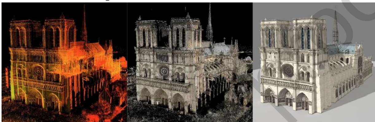
Fig. 4: LiDAR scanning played used in documenting and planning the restoration of Notre-Dame Cathedral, [13]
