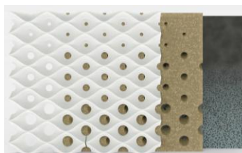
Figure 18: Phalanx Insulation System consists of three layers starting from the left: the shade layer, the air movement layer, and the capillary cooling layer. Source: (ECO Group IIT Roorkee: Phalanx-Insulation, 2021)
