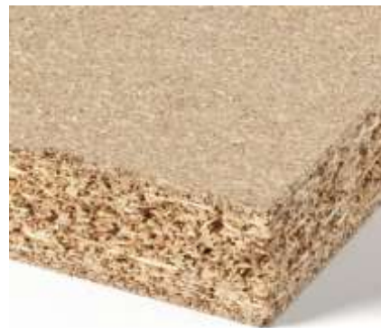
Figure (1) Low-density chipboard, manufactured from date palm waste
