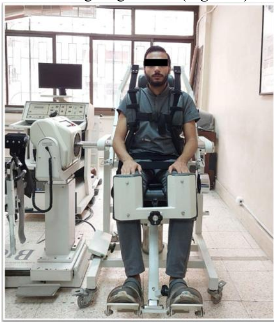
Figure (1): Testing position and stabilization.
