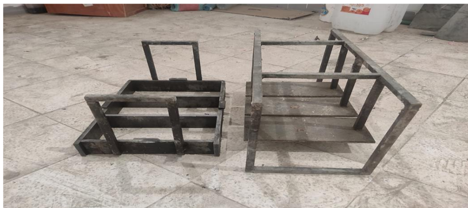
Fig. 3: Metal Mold for Cement Brick Fabrication
