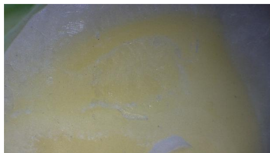
Figure (3b): Mixed failure shown in Group 2
