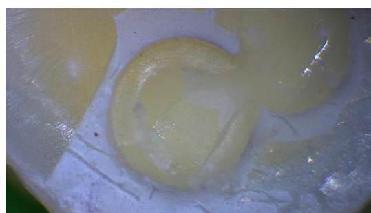
Figure (3c): Mixed failure shown in Group 3
