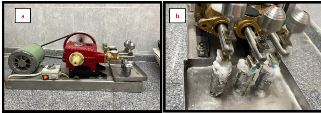
Figure 1 (a): A customized machine for simulation of tooth brushing, (b): Brushing cycles.
