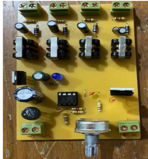
Figure 5.7: hardware of gate driver
