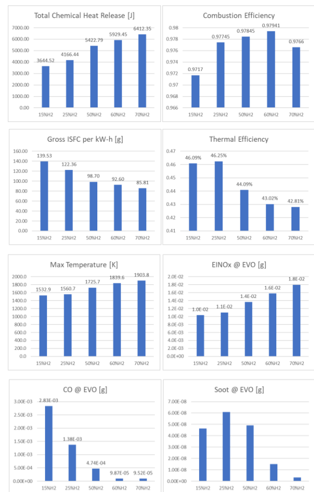
Fig. 16 Calculated total chemical heat release, Combustion Efficiency, Gross ISFC, thermal efficiency, maximum temperature, EINO x , CO, and soot at Hydrogen energy share at 15%, 25%, 50%, 60%, 70% at 2000 RPM
