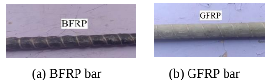
Figure 3. FRP NSM bars
