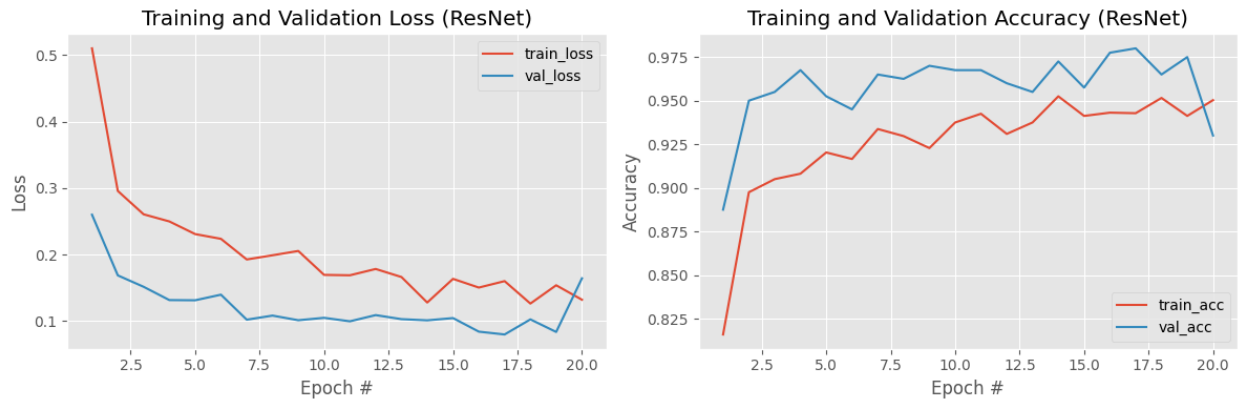
Figure 5. (Train-Validation) accuracy and loss through ResNet50-V2 pretrained model.
