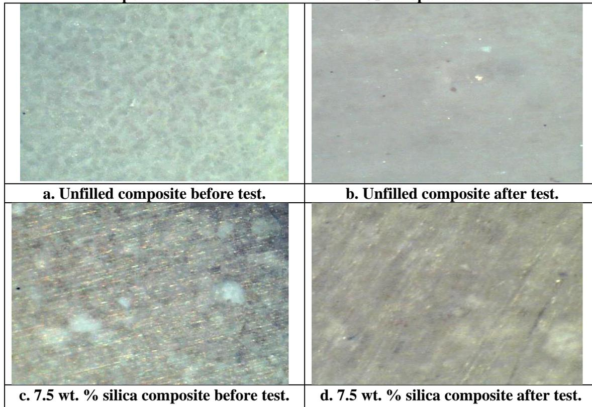
**Fig. 10** Photomicrographs of unfilled PMMA and PMMA/7.5 wt. % SiO<sub>2</sub> nanoparticles composites before and after test.
