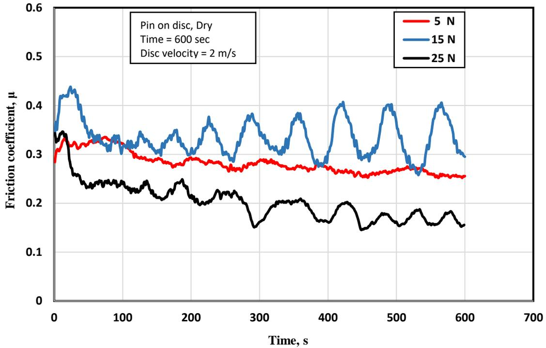
Fig. 4 The influence of the normal force on the friction coefficient for heat cured PMMA reinforced with 15 wt. % of SiO<sub>2</sub> nanoparticles.
