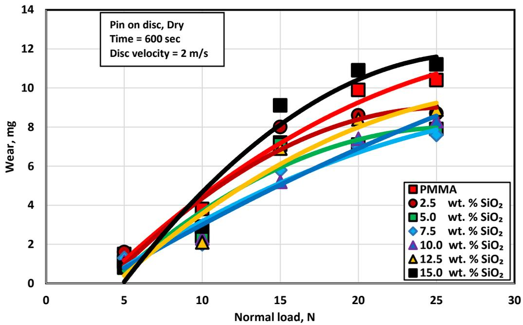
Fig. 5 The relation between the normal load and the wear for heat cured PMMA reinforced with different weight percentage of SiO<sub>2</sub> nanoparticles.
