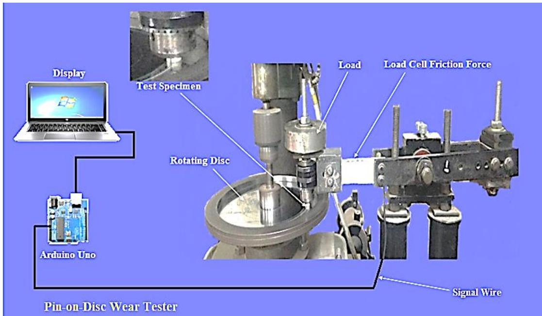
Fig. 1 General view for the pin-on-disc wear tester.
