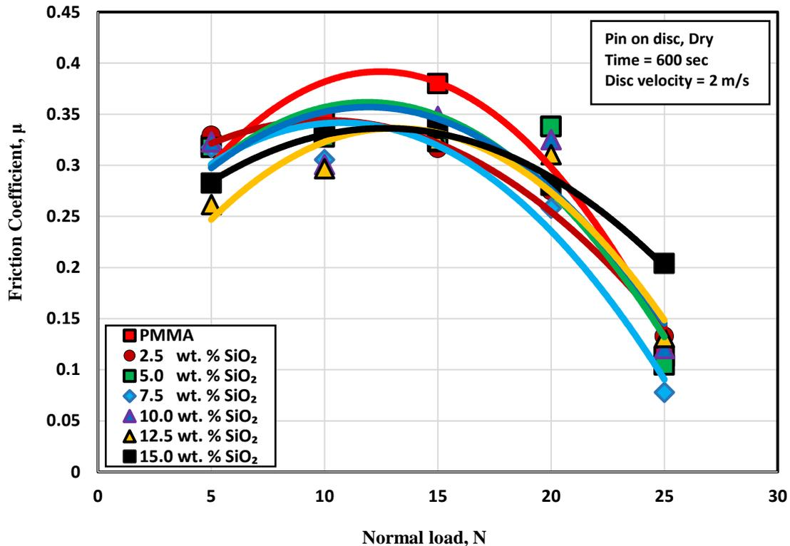
Fig. 6 The relation between the normal load and the average friction coefficient for heat cured PMMA reinforced with different wt. % of SiO<sub>2</sub> nanoparticles.
