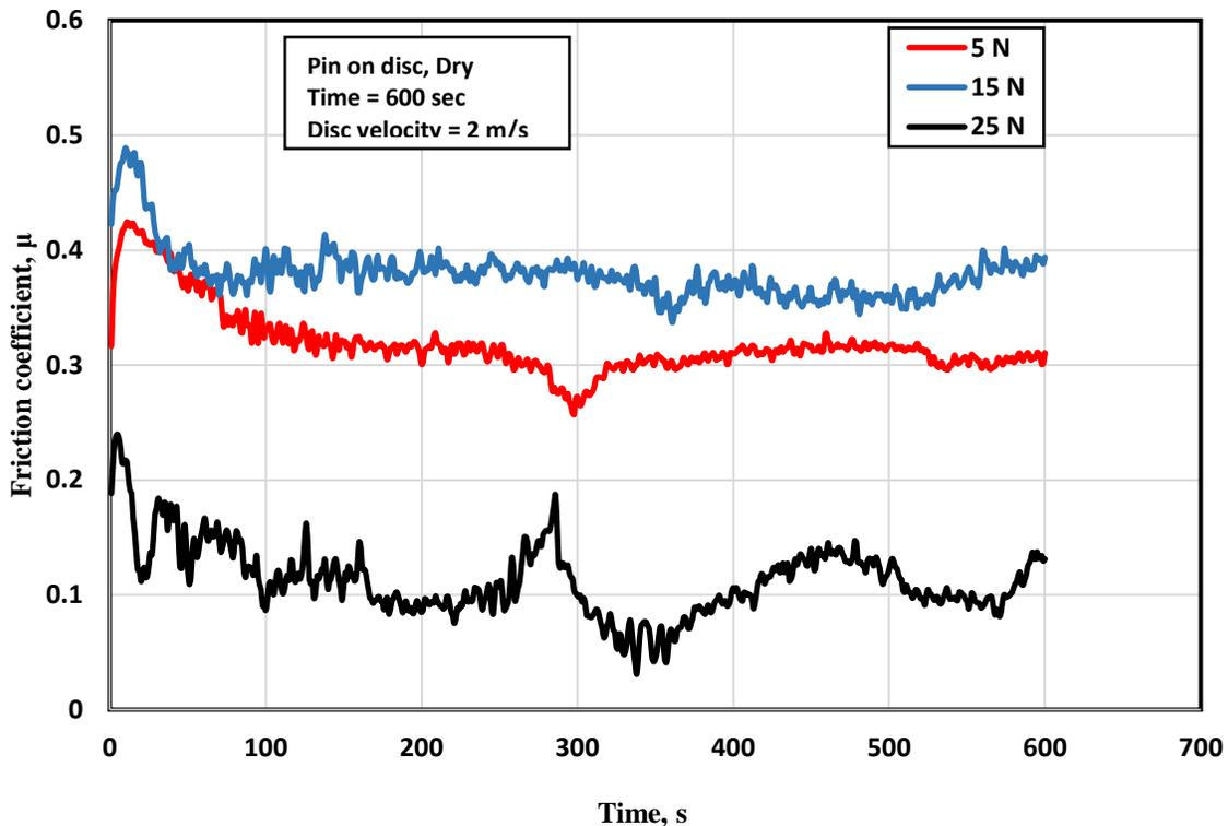
Fig. 2 The influence of the normal force on the friction coefficient for heat cured unfilled PMMA.
