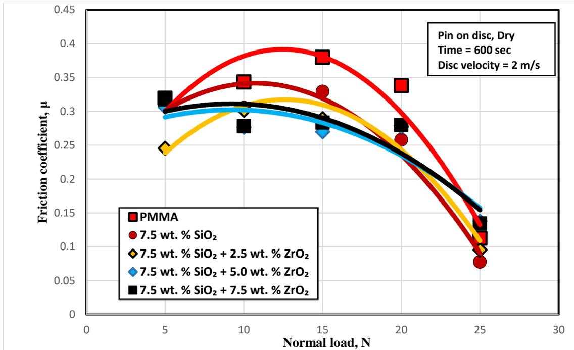
**Fig. 9** The relation between normal load and average friction coefficient for heat cured unfilled PMMA and (PMMA/7.5 wt. % SiO<sub>2</sub> nanoparticles) composites reinforced with different ZrO<sub>2</sub> nanoparticles content.
