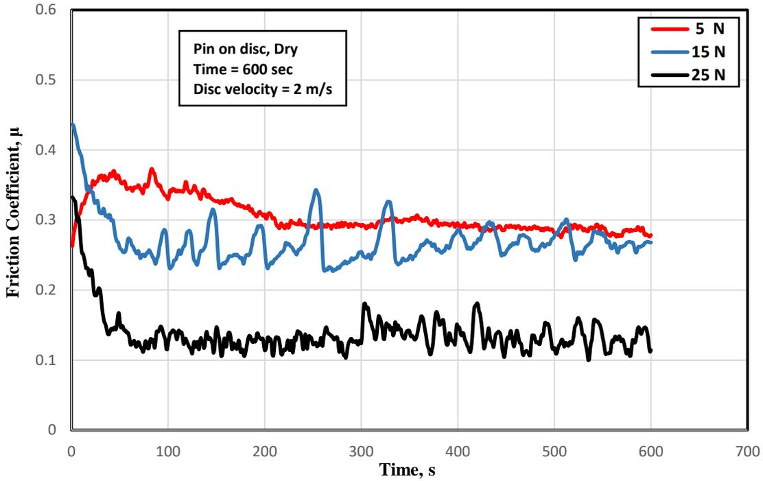
**Fig. 7** The influence of the normal force on the friction coefficient for heat cured PMMA reinforced with (7.5 wt. % SiO<sub>2</sub> and 5 wt. % ZrO<sub>2</sub>) nanoparticles.
