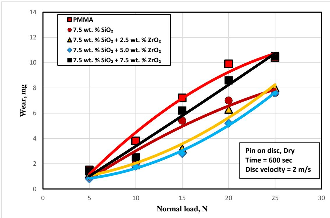
**Fig. 8** The relation between the normal load and the wear for heat cured unfilled PMMA and (PMMA /7.5 wt. % SiO<sub>2</sub> nanoparticles) composite reinforced with different content of ZrO<sub>2</sub> nanoparticles.
