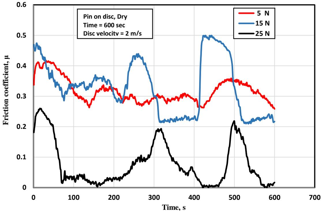
Fig. 3 The influence of the normal force on the friction coefficient for heat cured PMMA reinforced with 7.5 wt. % of SiO<sub>2</sub> nanoparticles.
