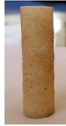
Fig. 5 test specimen filled by vegetables oil.
