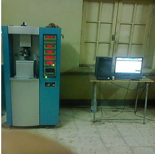
Fig. 1 Vertical universal friction and Wear testing machine [MM-W1A].
