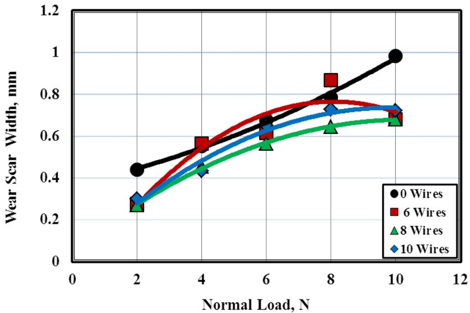
Fig. 18 Wear displayed by the scratch of HDPE reinforced by 0.4 mm diameter copper wires and annealed at 90 °C.
