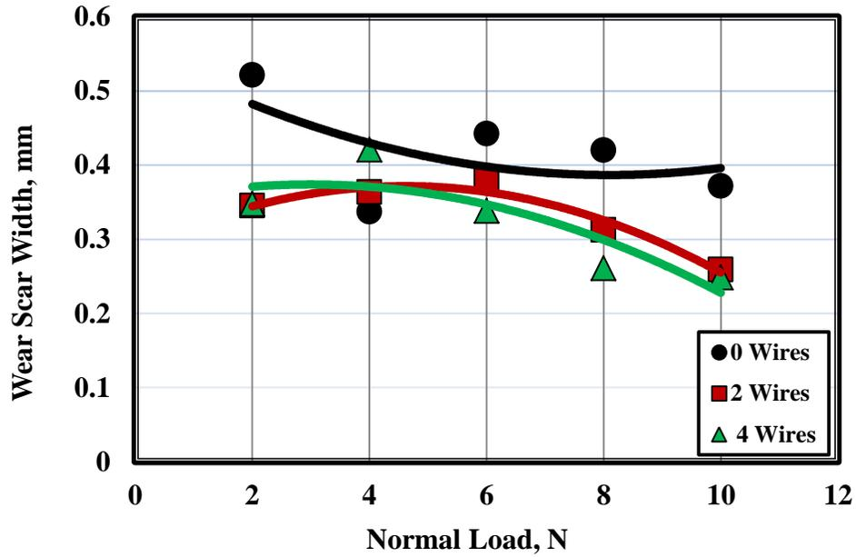
Fig. 21 Wear displayed by the scratch of HDPE reinforced by 0.4 mm diameter copper wires treated by tempering at 110 °C.
