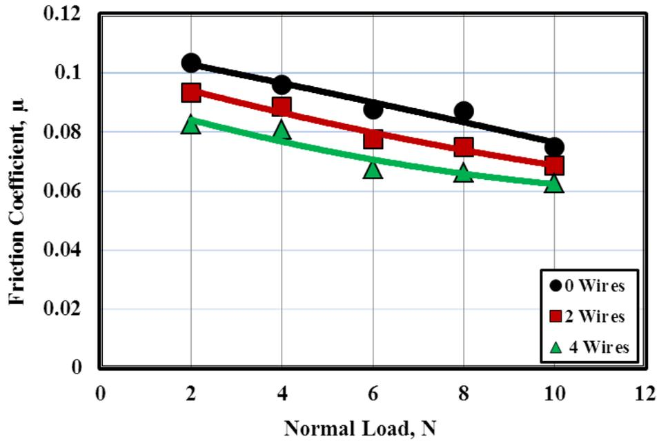
Fig. 13 Friction coefficient displayed by the scratch of HDPE reinforced by 0.4 mm diameter copper wires and tempered at 110 °C.
