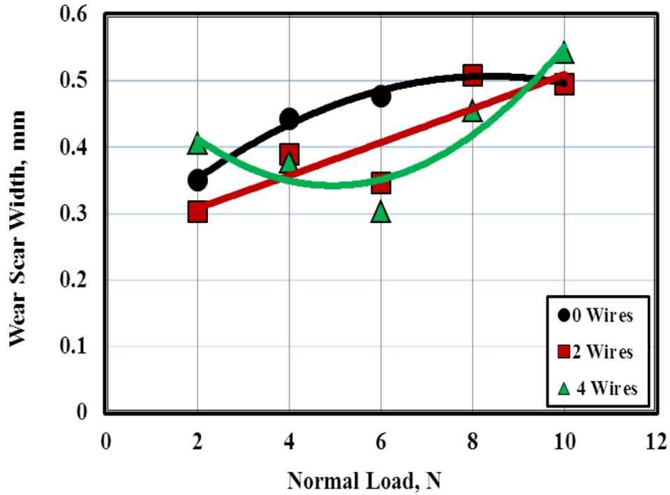
Fig. 19 Wear displayed by the scratch of HDPE reinforced by 0.4 mm diameter copper wires hardened at 120 °C.
