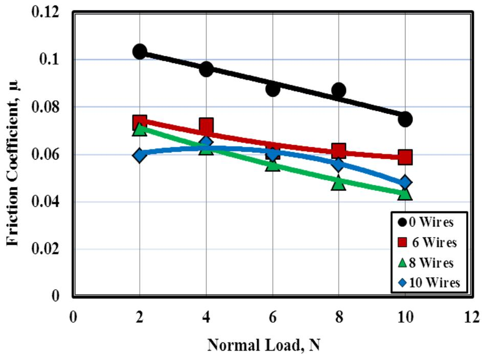
Fig. 14 Friction coefficient displayed by the scratch of HDPE reinforced by 0.4 mm diameter copper wires treated by tempering at 110 °C.
