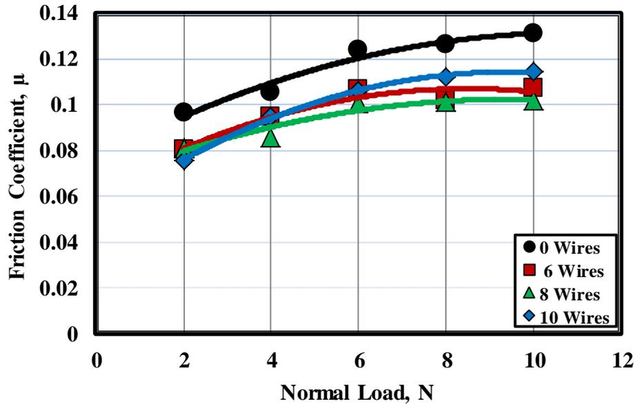
Fig. 8 Friction coefficient displayed by the scratch of HDPE reinforced by 0.4 mm diameter copper wires.
