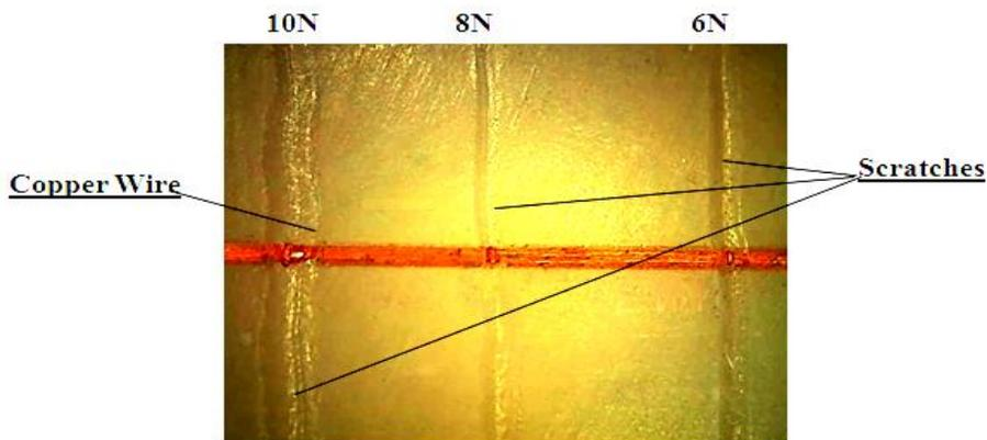
**Fig. 6 scratch tests on the surface of the test specimen.**
