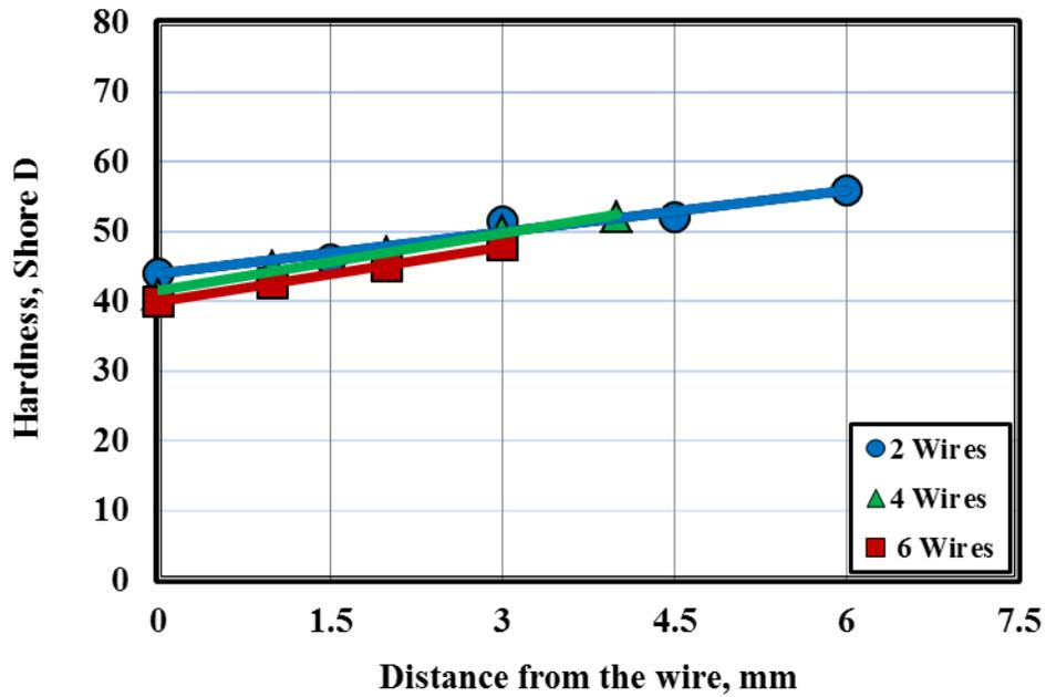
**Fig. 26** Hardness distribution on the surface of tempered HDPE composites reinforced by 0.4 mm diameter copper wires.
