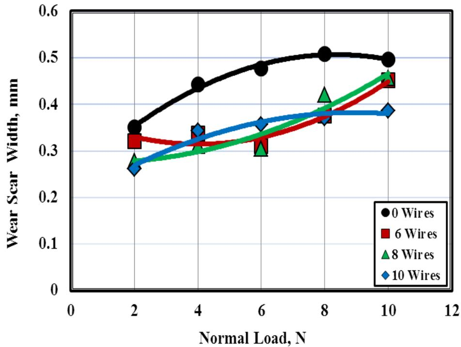
Fig. 20 Wear displayed by the scratch of HDPE reinforced by 0.4 mm diameter copper wires and hardened at 120 °C.
