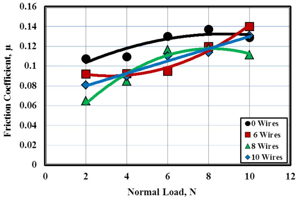
Fig. 10 Friction coefficient displayed by the scratch of HDPE reinforced by 0.4 mm diameter copper wires and annealed at 90 °C.
