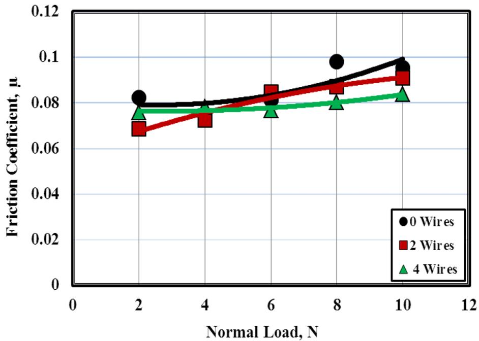
Fig. 11 Friction coefficient displayed by the scratch of HDPE reinforced by 0.4 mm diameter copper wires and hardened at 120 °C.
