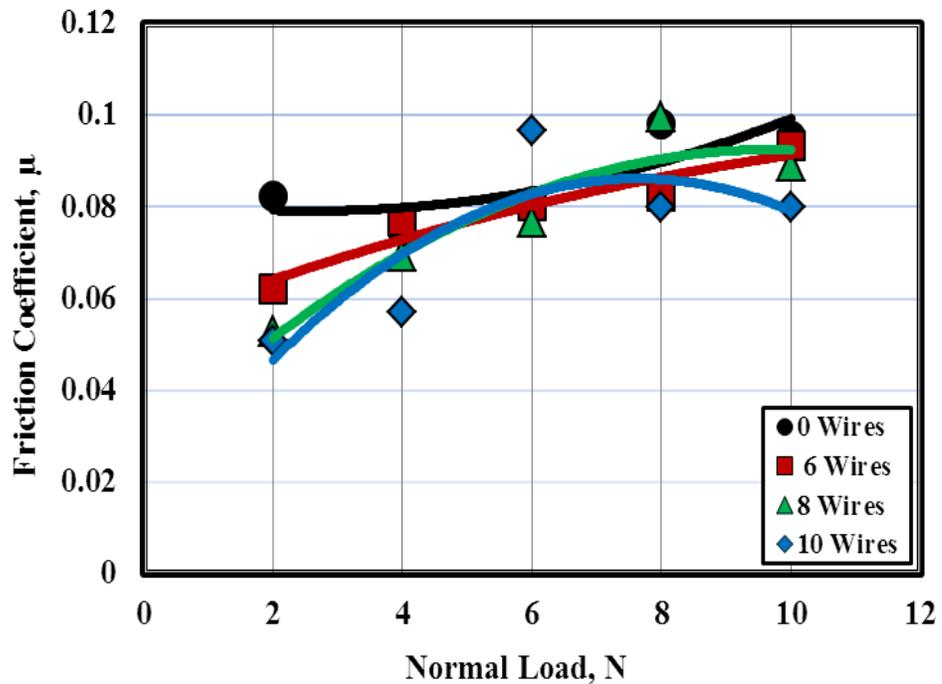
Fig. 12 Friction coefficient displayed by the scratch of HDPE reinforced by 0.4 mm diameter copper wires and hardened at 120 °C.
