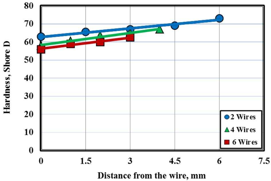
Fig. 23 Hardness distribution on the surface of HDPE composites reinforced by 0.4 mm diameter copper wires.
