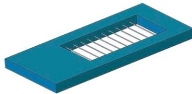
Fig. 1 Molding die of the test specimens.
