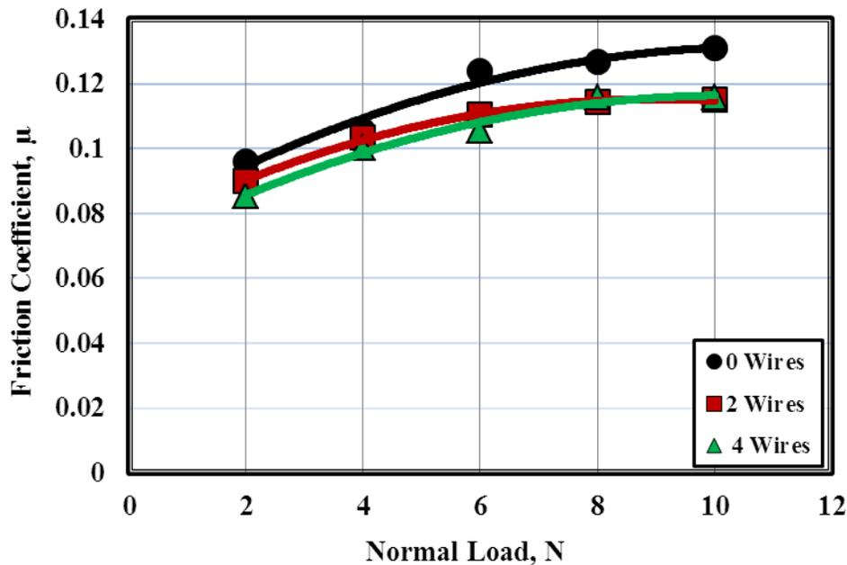
Fig. 7 Friction coefficient displayed by the scratch of HDPE reinforced by 0.4 mm diameter copper wires.
