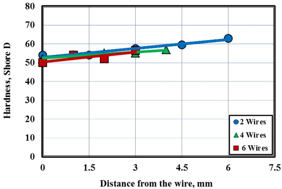
Fig. 24 Hardness distribution on the surface of annealed HDPE composites reinforced by 0.4 mm diameter copper
