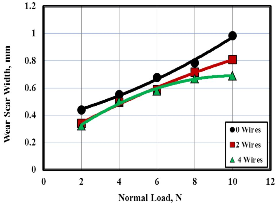
Fig. 17 Wear displayed by the scratch of HDPE reinforced by 0.4 mm diameter copper wires and annealed at 90 °C.
