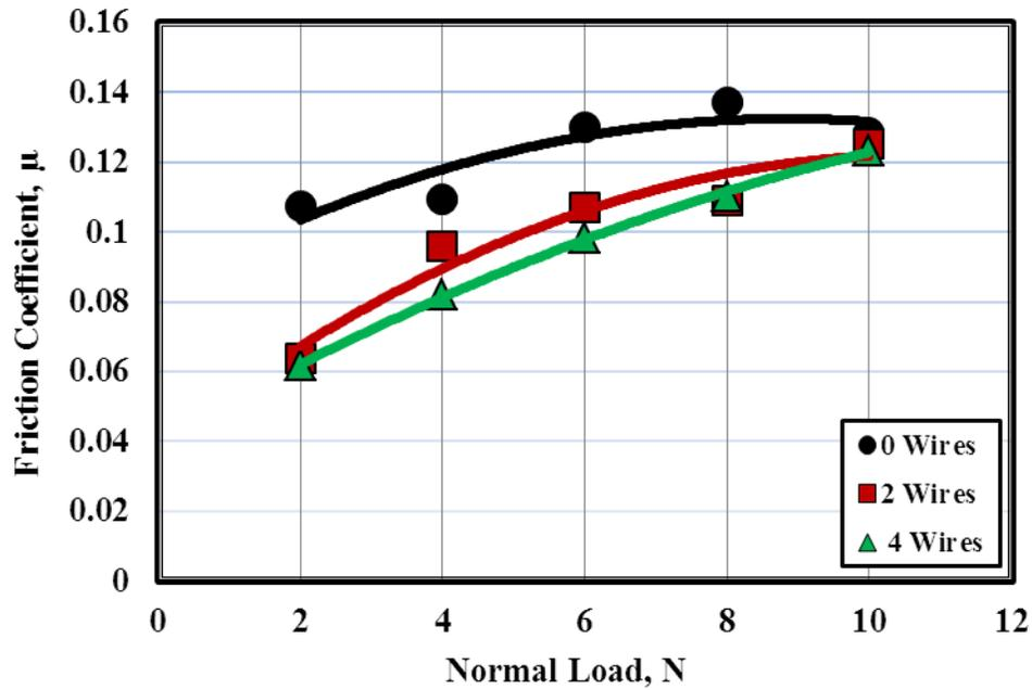
Fig. 9 Friction coefficient displayed by the scratch of HDPE reinforced by 0.4 mm diameter copper wires and annealed at 90 °C.
