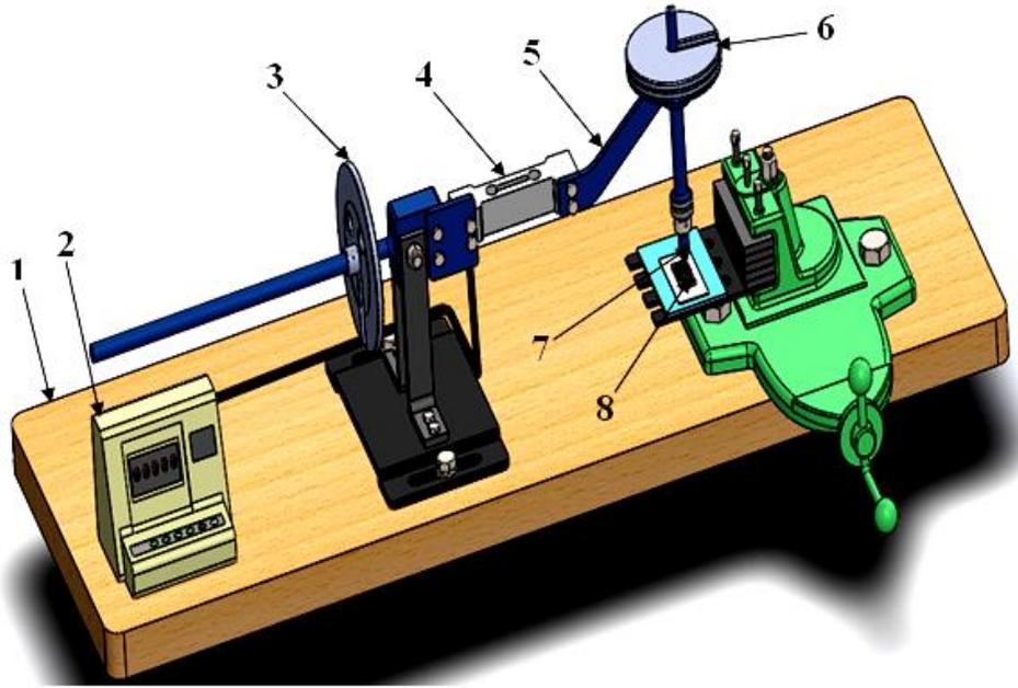
**Fig. 4 Arrangement of scratch test rig; 1. Base, 2. Friction Force Screen, 3. Counter Weight, 4. Load Cell, 5. Loading Lever, 6. Normal Loads, 7. Scratching tool, 8. Test Specimen.**
