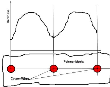
Fig. 27 Hardness change due to the caused by copper wires. [4].
