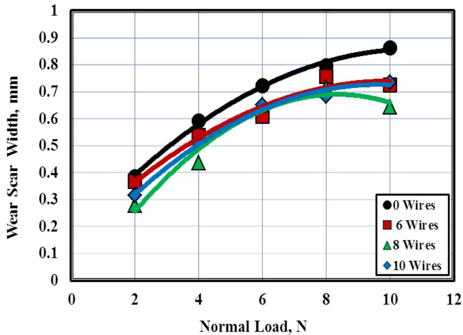
Fig. 16 Wear displayed by the scratch of HDPE reinforced by 0.4 mm diameter copper wires.
