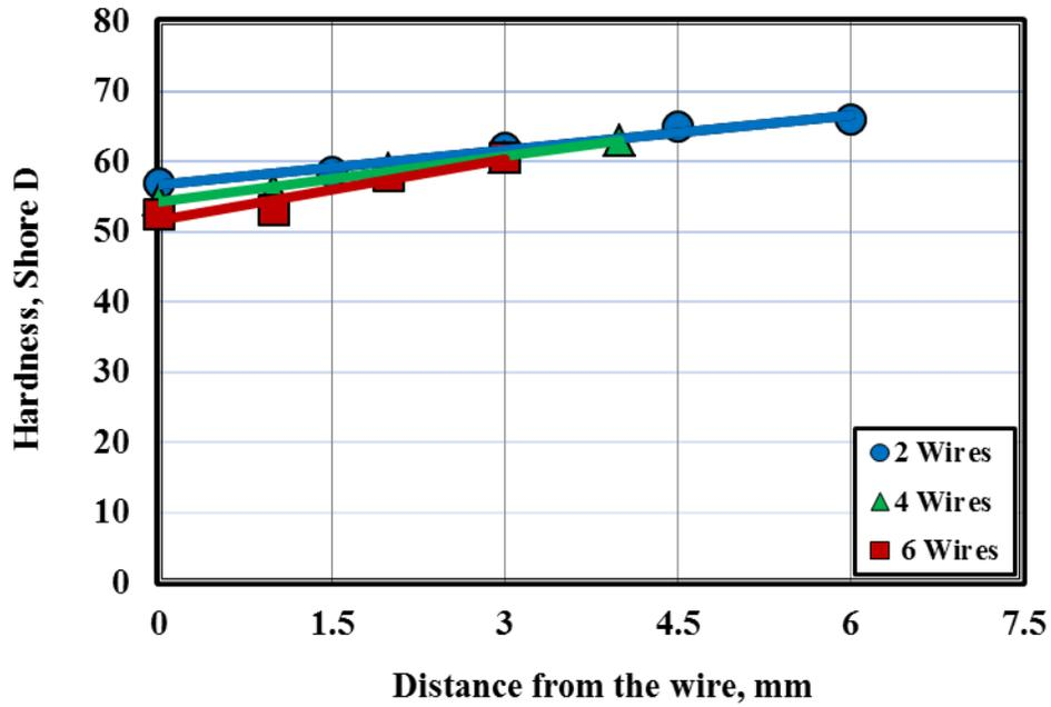
**Fig. 25** Hardness distribution on the surface of hardened HDPE composites reinforced by 0.4 mm diameter copper wires.
