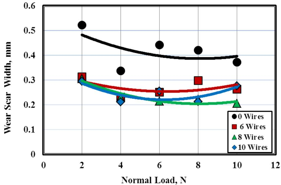
Fig. 22 Wear displayed by the scratch of HDPE reinforced by 0.4 mm diameter copper wires treated by tempering at 110 °C.
