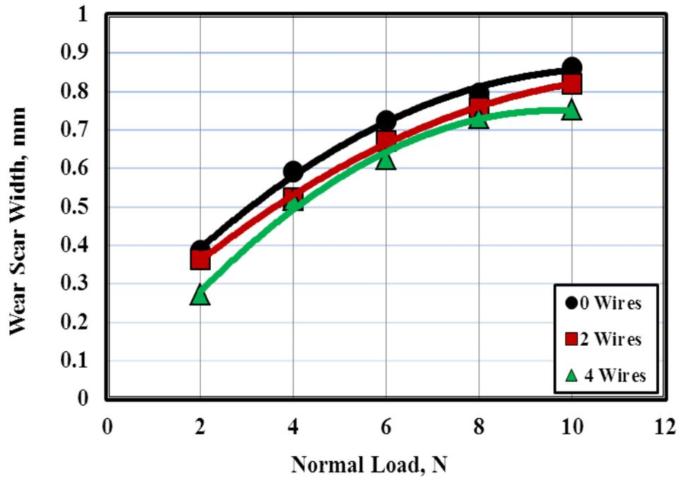
Fig. 15 Wear displayed by the scratch of HDPE reinforced by 0.4 mm diameter copper wires.
