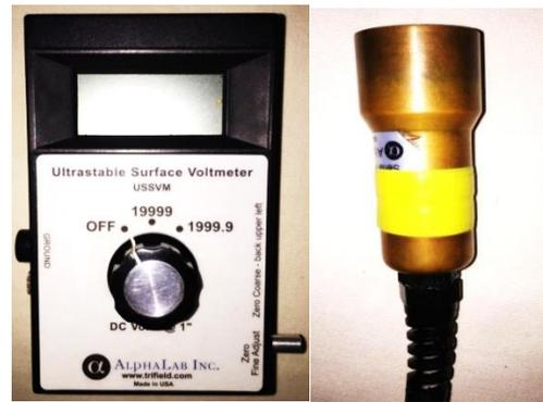
Fig. 2 ESC measurement device.
