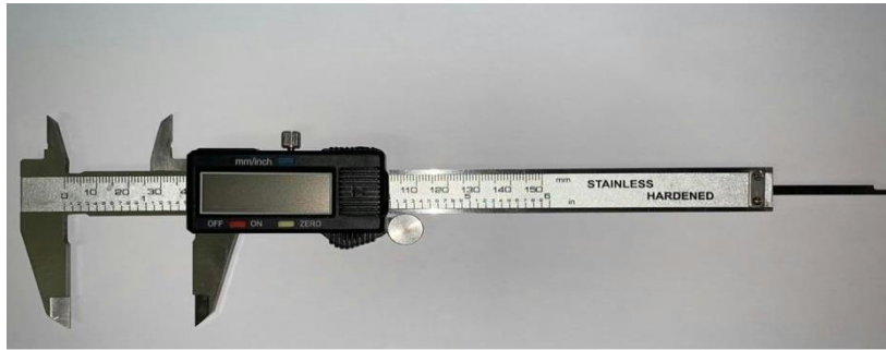
Fig I: Showing a Vernier digital calipers with an accuracy of 0.1mm.
