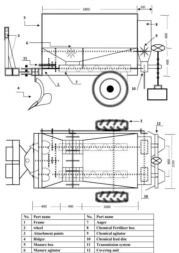
Fig. 2. A sketch of the manufactured machine
