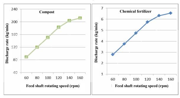
Fig. 3. Effect of feed shaft rotating speed on fertilizer discharge rate
