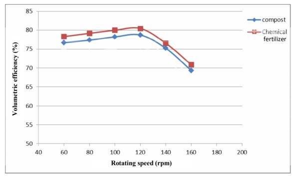
Fig. 4. Effect of feed shaft rotating speed on volumetric efficiency
