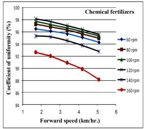
Fig. 6. Effect of the forward speed on coefficient of uniformity of fertilizers distribution at different rotating speed
