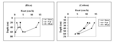
Fig.(5): Hydraulic conductivity (K<sub>sat</sub>) of the studied profiles as affected by rice and cotton cultivation for 5 and 10 years.
