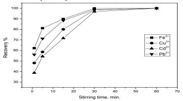
Fig. 5. The effect of stirring time on the recovery of different metal ions.
