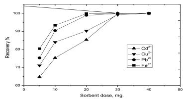
Fig. 6. The effect of sorbent dose on the recovery of different metal ions.
