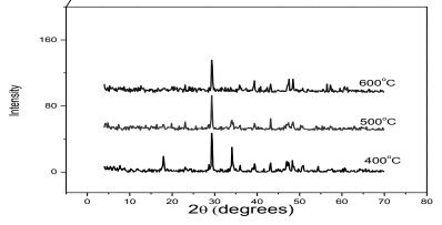
Fig.1. XRD pattern of nano-CaO sorbent.
