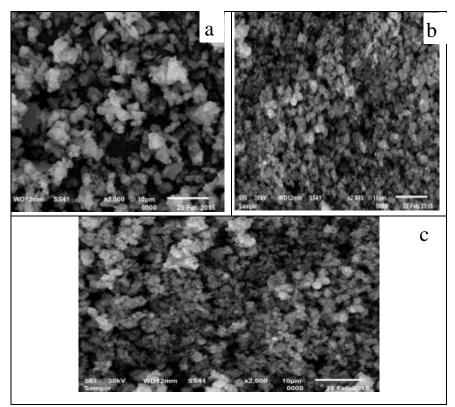
Fig. 3. SEM images of nano-CaO sorbent calcinated at a) 400°C, b) 500°C, and c) 600°C.
