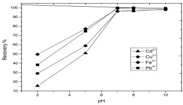
Fig. 4. The effect of pH on the recovery of different metal ions.
