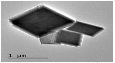
Fig. 2. TEM image of nano-CaO sorbent calcinated at 500°C.
