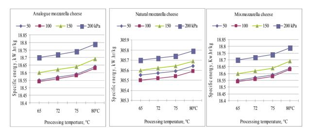
Fig.7. Effect of processing temperature on the specific energy for producing analogue, natural and mix mozzarella cheese
