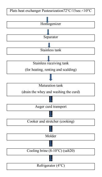
Fig. 2: Flow chart of equipments used in natural mozzarella cheese production
