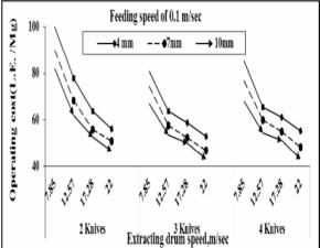
Fig. 7. Effect of extracting drum speed on operational cost under different clearances, and knife number using feeding speeds of 0.05, 0.1 and 0.15 m/sec.
