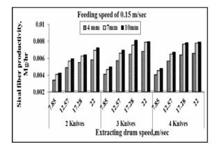
Fig. 4. Effect of extracting drum speed on sisal fiber productivity under different clearances, and knife number using feeding speeds of 0.05, 0.1 and 0.15 m/sec.
