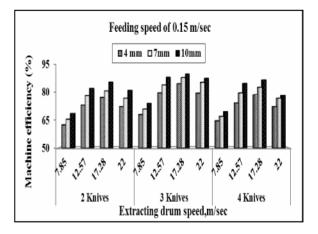
Fig. 3. Effect of extracting drum speed on machine efficiency under different clearances, and knife number using feeding speeds of 0.05, 0.1 and 0.15 m/sec. leads to increase machine efficiency from 71.81 to 74.22, from 86.23 to 88.63, from 89.92 to 90.34, and from 86.32 to 88.05%, under the same previous conditions, at clearances between the knives and the feeding drum of 10mm and knife number of 3.
