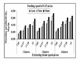
Fig. 2. Effect of extracting drum speed on machine productivity under different clearances, and knife number using feeding speeds of 0.05, 0.1 and 0.15 m/sec.
