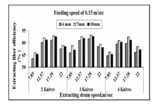
Fig. 5. Effect of extracting drum speed on extracting fiber efficiency under different clearances, and knife number using feeding speeds of 0.05, 0.1 and 0.15 m/sec.
