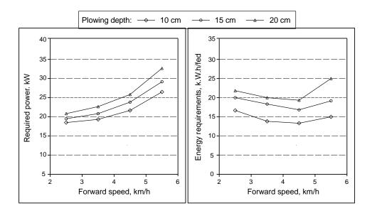
Fig. (8): Effect of machine forward speed on required power and energy requirements under different plowing depths.
