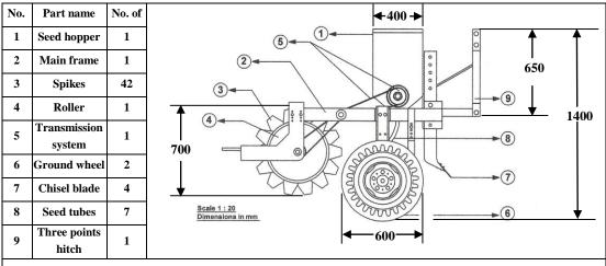
Fig.1: Side view of the manufactured combination machine.
