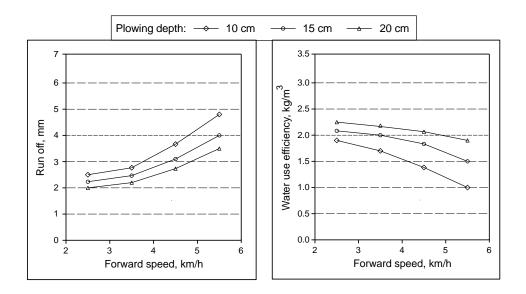
Fig. (6): Effect of machine forward speed on runoff and water use efficiency under different plowing depths.
