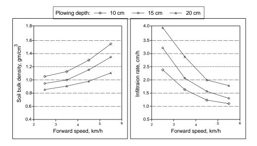
Fig. (4): Effect of machine forward speed on soil bulk density and infiltration rate under different plowing depths.
