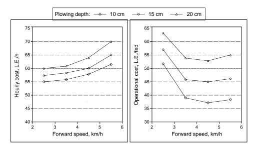
Fig. (9): Effect of machine forward speed on hourly cost and operational cost under different plowing depths.
