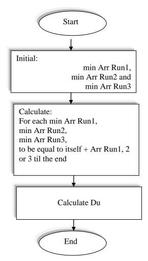
Fig4. Flow chart for calculating distribution uniformity (Du)
