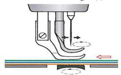
Figure (4): Unison feed mechanism
