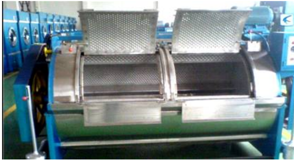
Figure (3) Side Loading Cellulase Washing Machine
