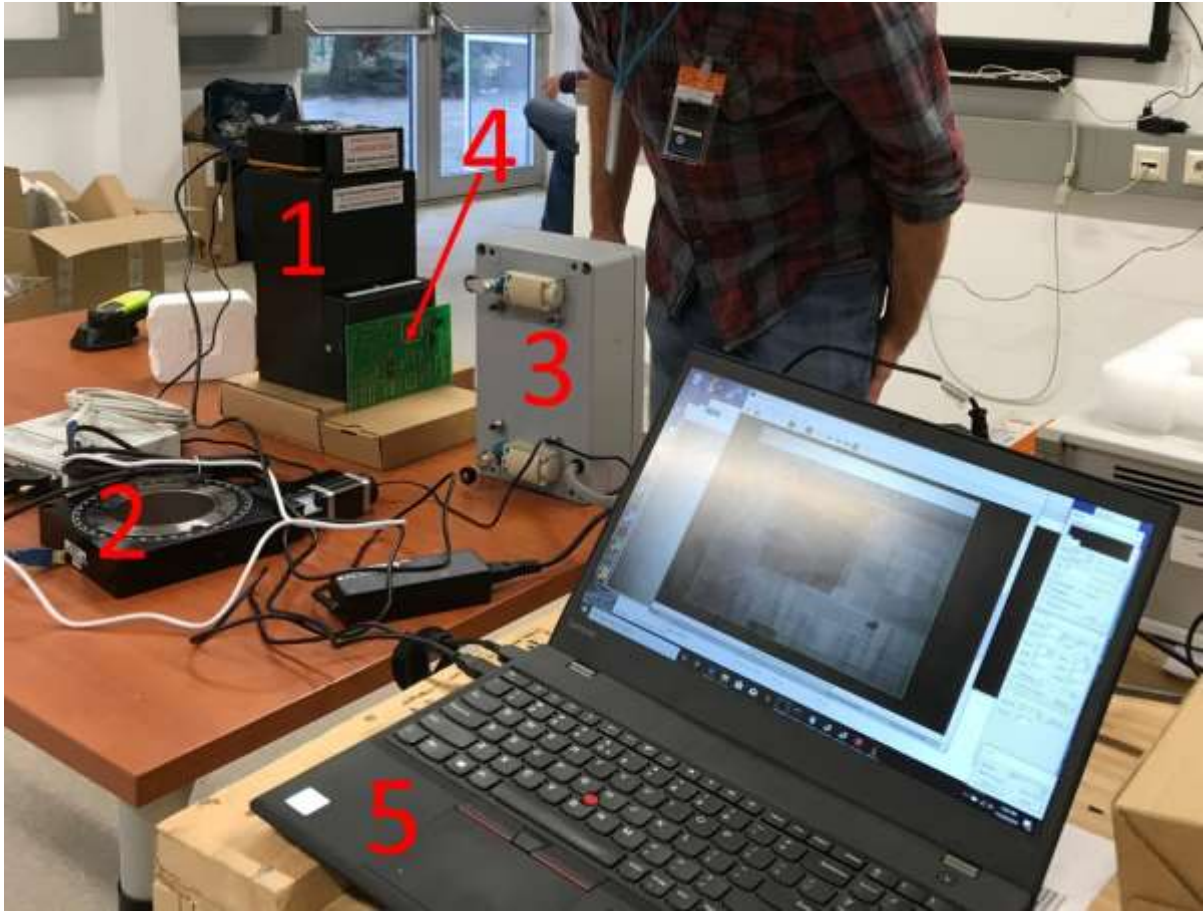
Figure 5: Testing of the dual neutron / X ray imaging system. 1: camera box; 2: rotating stage (not in use in this image); 3: X ray source; 4: sample; 5: computer control.
