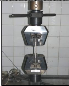
Figure 1. The placement of the specimen before tensile loading.
