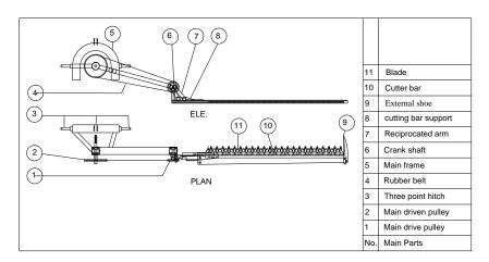
Fig. (1): The components of the original mower
