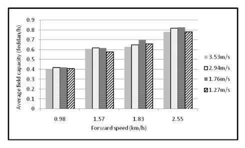
Fig (8): The relation between Forward speed and field capacity in different conveyer linear speed.
