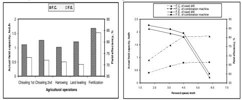
Fig. (7):Effect of different Fig. (8):Effect of forward speedagricultural operations on field on field capacity and fieldfield capacity and fieldcapacity and field efficiencyefficiency
