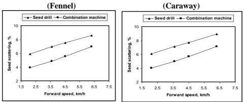
Fig. (4): Effect of forward speed on seed scattering for fennel and caraway under seed drill and developed combination machine
