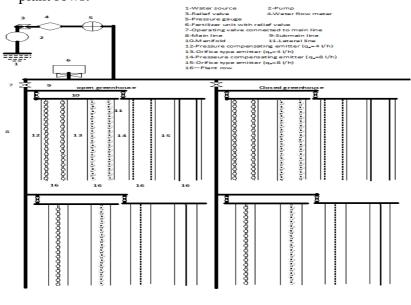
Figure (1) represents the schematic diagram of the experimental trickle irrigation system constructed in each greenhouse.
